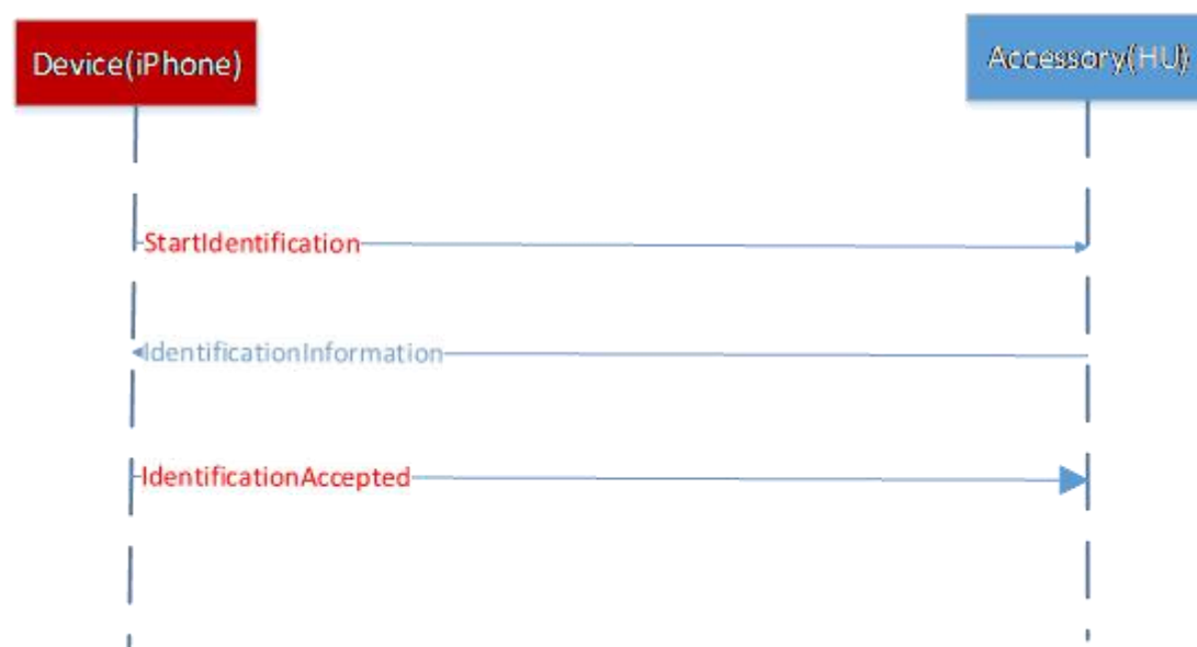
Figure 6.1-18: Accessory Identification Sequence Diagram
